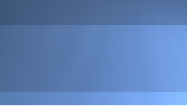
Figure 2: Image of a stroboscopic flash at 100Hz with a rolling shutter camera.
