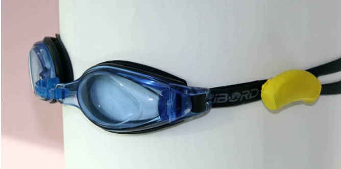
Fig. 1. The modified waterproof ear-worn Activity Recognition (e-AR) sensor mounted on the swimmer's goggles.
