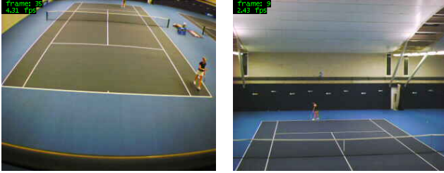
Figure 5. Left: near side of the court as seen by the VSN node with a 3.6mm focal length optic. Right: far side as seen with a 6.5mm focal length.
