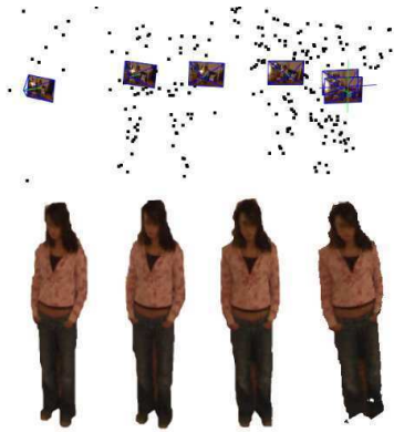
Figure 1. Extrinsic parameters estimated by the proposed method and a series of segmented silhouettes. The final silhouette is generated using image-based rendering.
